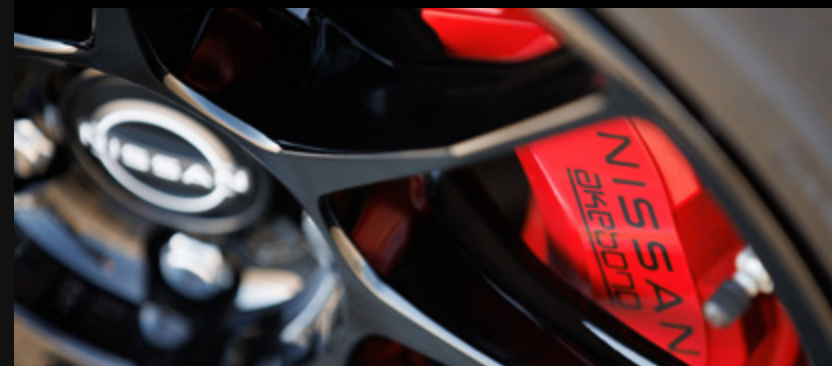
19" x 10J" front & 19" x 10.5J" rear gloss black painted forged alloy wheels by RAYS®
